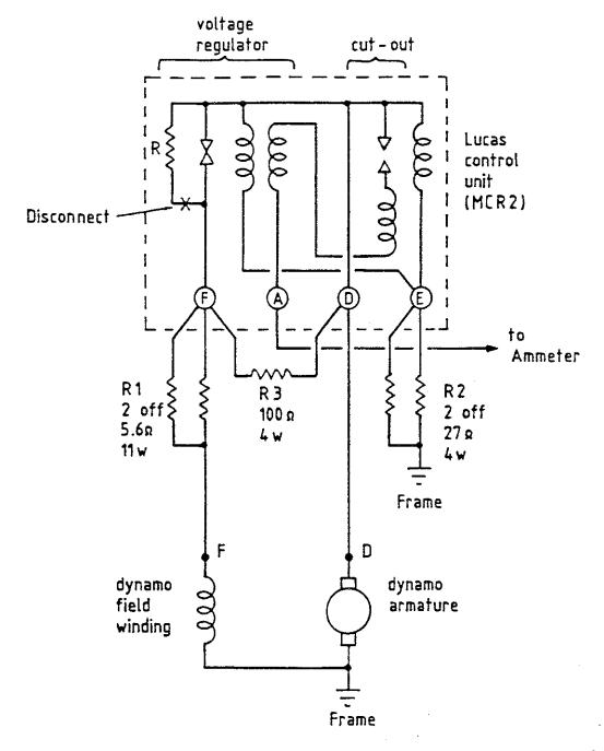
were open. Unfortunately, I now realised that there was no alternative to a minor internal modification to the control unit. This consisted of disconnecting one end of resistor R, as indicated by X in the diagram, and insulating the floating lead. A substitute resistor R3, twice the value of the original, was connected externally between the F and D terminals.
