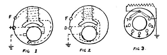
Fig. 2 is of course, the usual two brush dynamo, with earthed neg. brush coupled to one end of field winding. The other end of the field being brought out at terminal F.
