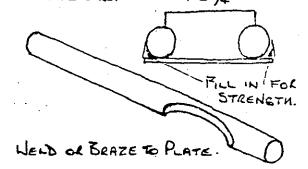
HAKE TWO 1/2" SILVER STEEL SHAFTS. GRIND HALFWAY THROUGH (1/4"), CLEARANCE FOR RELEASE BEARING O.D. LENGTH TO BE 33/4" PLUS LEVER NIDTH, PLUS CIRCLIP.
