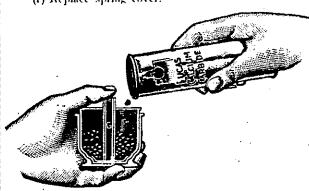
To start the Generator when charged with water and carbide, turn the Regulator B, and it should be ready for lighting in a few seconds. If it does not start readily, either the burner is stopped or the Regulator has not been turned far enough to allow sufficient water to drop down to the carbide. Nearly every trouble with Acetylene Lamps may be avoided by strict cleanliness, and omission in this direction is sure to cause difficulty.
