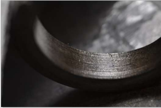
Inside surface of 1911 main bearing inner ring showing turned surface before hardening
