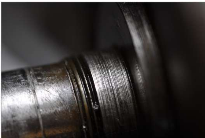
Mounting surface of 1911 crank main bearing inner ring mounting diameter showing turned finished then hardened
